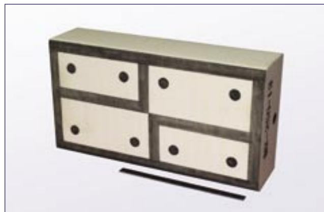
Figure 3.8-3. A typical foam projectile, which has marks for determining position and velocity as well as blackened outlines for indicating the impact footprint.
