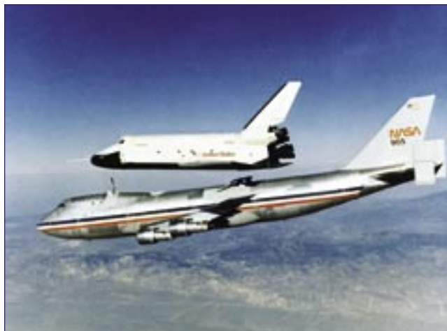
Figure 1.3-1. The first Orbiter was Enterprise, shown here being released from the Boeing 747 Shuttle Carrier Aircraft during the Approach and Landing Tests at Edwards Air Force Base.
