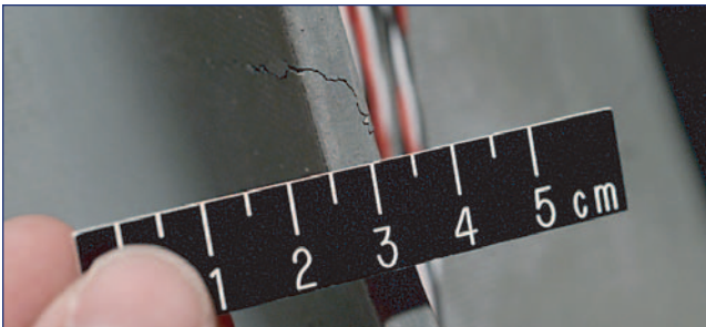
Figure 3.8-6. A 5.5-inch crack on the outboard portion of RCC Panel 6 during testing.
