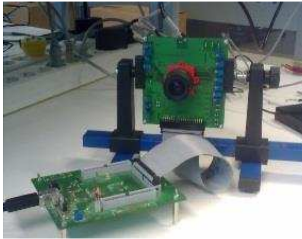
Figure 3—Experimental setup: vision sensor and data logger.
