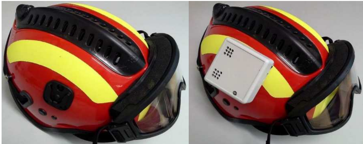
Figure 4. Helmet module prototype integration: original firefighter helmet (on the left) and helmet equipped with monitoring hardware (on the right).
