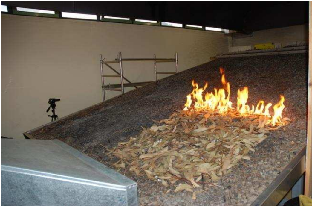
Figure 1. A fire-spread sustainability trial in the combustion table.
