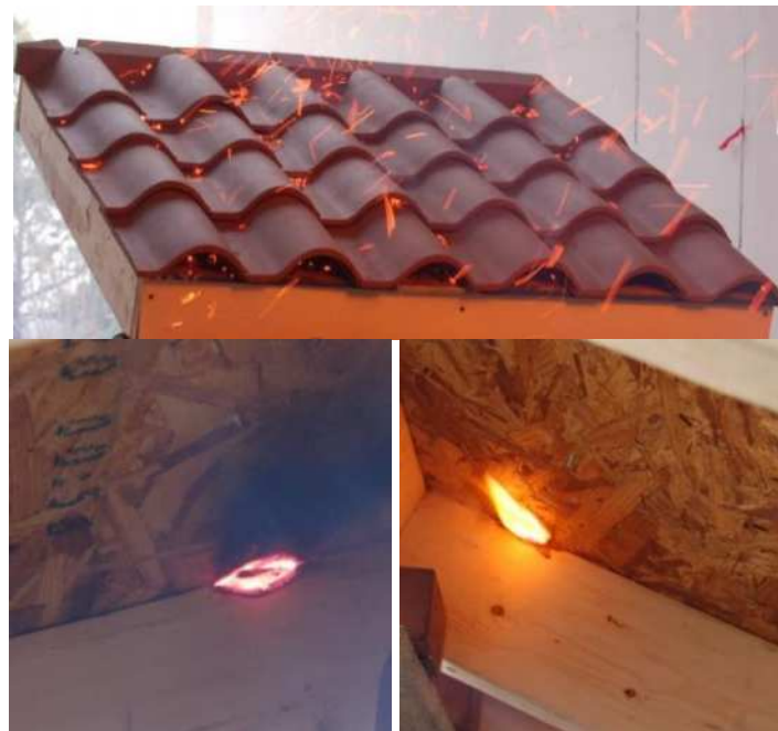
Figure 4. Images of experiments conducted using oriented strand board/ceramic tile (OSB/CT) without bird stops installed [11]. Intense smoldering ignition (SI) was observed within the OSB base layer and eventually flaming ignition (FI) was observed. The wind tunnel speed was 7 m/s and the Firebrand Generator was located 2.0 m from the CT roofing assembly. The dimensions of the roof assembly were 122 cm by 122 cm.
