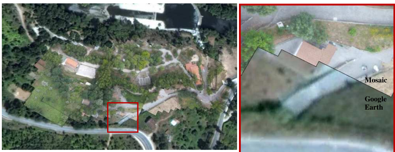
Figure 4. Left: High-resolution mosaic, constructed from aerial images acquired by a quadcopter over the camping site of Côja, overlaying Google Earth. Right: Zoom of the area indicated in red in the image on the left.
