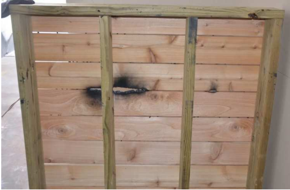
Figure 2. Picture of the underside of the decking assembly (cedar); overall view [10].
