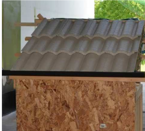
Figure 5. Concrete Tile Roofing Assembly (profiled tile) Exposed to Wind-Driven Firebrand Showers. The dimensions of each tile were 420 mm long by 320 mm wide. The Height, from the Wind Tunnel Floor to the Base of the Gutter of Roof Deck was 1250 mm [12].
