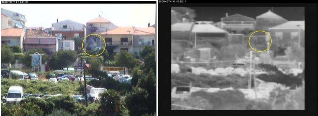
Figure 2. Smoke visibility during typical hot summer day in visible spectra (left) and far IR spectra (right)
