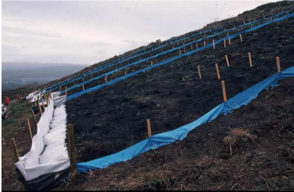
Figure 4. View of the macro-plots delimited by geotextile fabrics to measure post-fire erosion.
