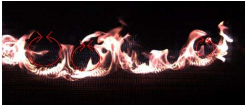
Figure 1. A high speed color photographic image of spreading flame over artificially made cardboard fuelbeds (Finney, Forthofer et al. 2013).
