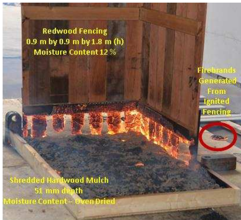
Figure 8 Redwood fencing (inside corner section), exposed to wind-driven firebrand showers at 8 m/s from the NIST Dragon. The firebrands produced smoldering ignition in the shredded hardwood mulch bed (foreground; depth 51mm), this transitioned to flaming ignition in the mulch, and the redwood fencing was subsequently ignited by the mulch. Shredded hardwood mulch was intended to represent various fuels that are adjacent to fencing in the Wildland-Urban (WUI). As the redwood fence continued to burn, firebrands were generated with large projected area and low mass, and were blown downstream (far right).
