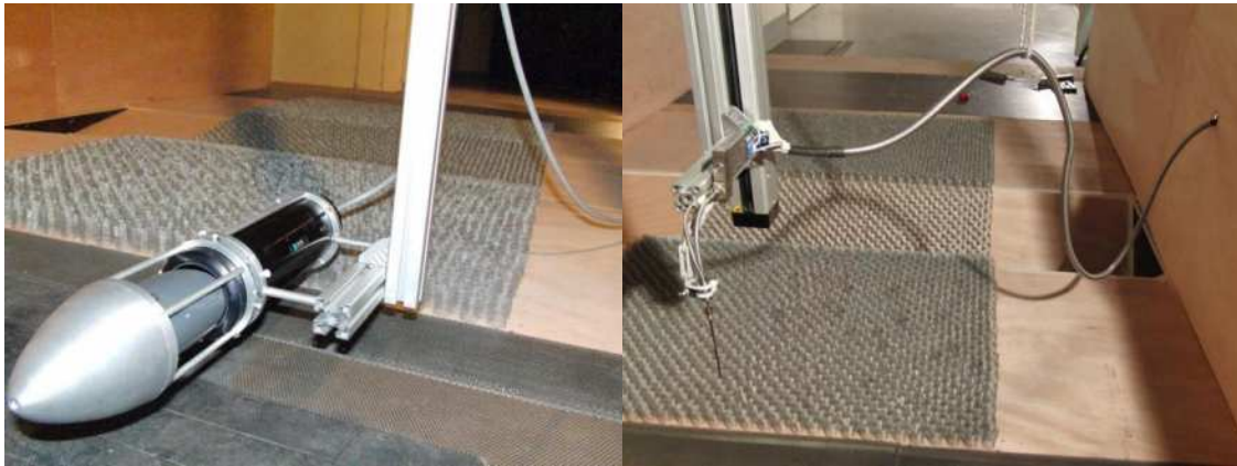
Figure 4. LDV on the left and FID on the right above the V-shaped forest model
