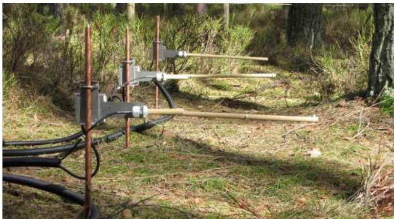
Figure 1. Arrangement of fuel moisture sticks at the forest climate station Altdorf.
