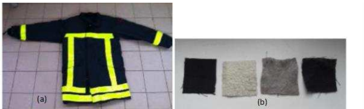
Figure 1. Standard fire protective jacket (a). Samples of the different layers involved (b)
