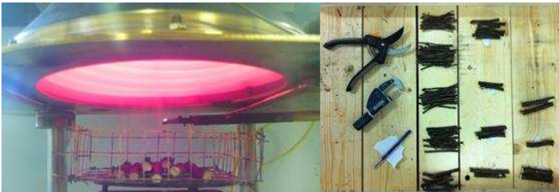
Figure 1. a) Experimental device b) Twigs of Cistus Monspeliensis used as fuel
