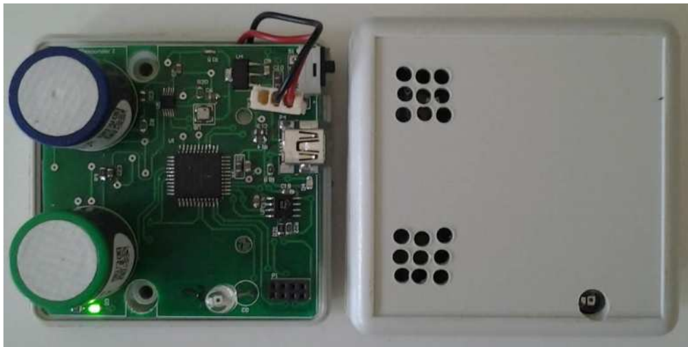
Figure 3. Helmet module prototype: hardware picture (on the left) and its integration on suitable box (on the right).
