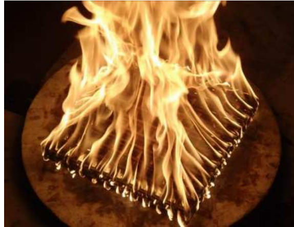
Fig 4. Crib with l/b = 48 burning from the outside edges inward.
