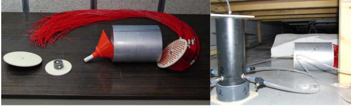
Figure 3. The two photographs depict the distribution device of ethane placed under the model
