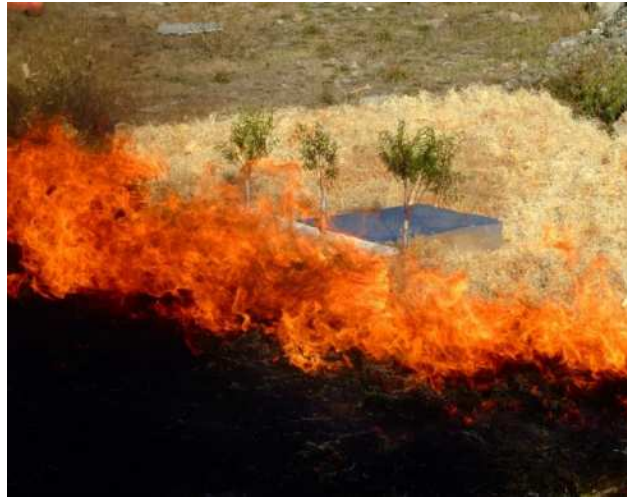
Figure 2. Differential mass loss prototype in field conditions
