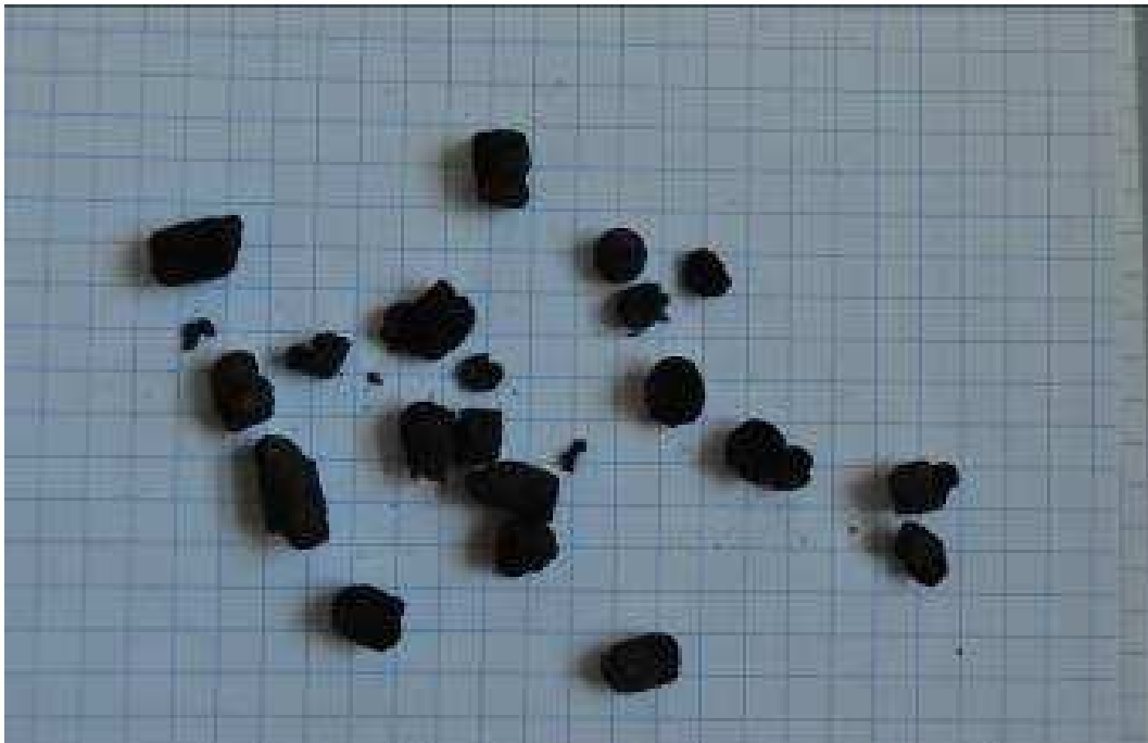
Figure 4. An example of firebrand dimensions obtained in the tests are showed in a 3 mm x 3 mm grid
