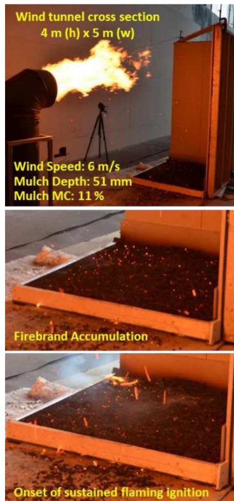
Figure 7. Image of 1.2 m by 1.2 m by 51 mm (depth) shredded hardwood mulch bed at 11 % MC exposed to continuous wind-driven firebrand showers. The re-entrant corner, with dimensions of 1.2 m by 1.2 m by 2.44 m high, was lined with gypsum board to investigate the ignition of the mulch bed itself; the ability of the mulch bed to ignite the wall assembly was not considered [14].
