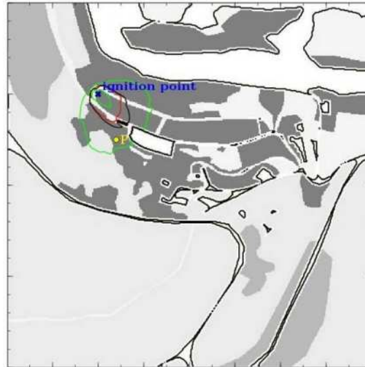
Figure 6. Forecast of the fire front in the CP of Coja after 4 hours of ignition: deterministic mean (black); stochastic mean (red); error area with 95% CI (between green lines).
