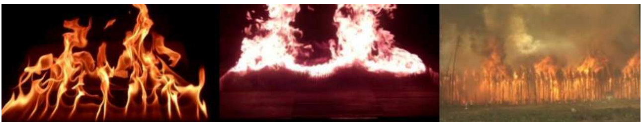
Figure 1. Photos demonstrating the scales over which coherent streaks and flame towers have been observed. (a) Inclined gas burner, L_f \approx 0.2 m, (b) Comb burn experiments in 3×3 m wind tunnel, L_f \approx 2 m, and (c) Canadian Crown fire experiments, L_f \approx 30 m (Clark et al. 1999).
