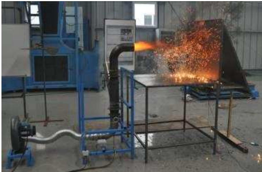
Figure 1. Firebrand Generator Device
