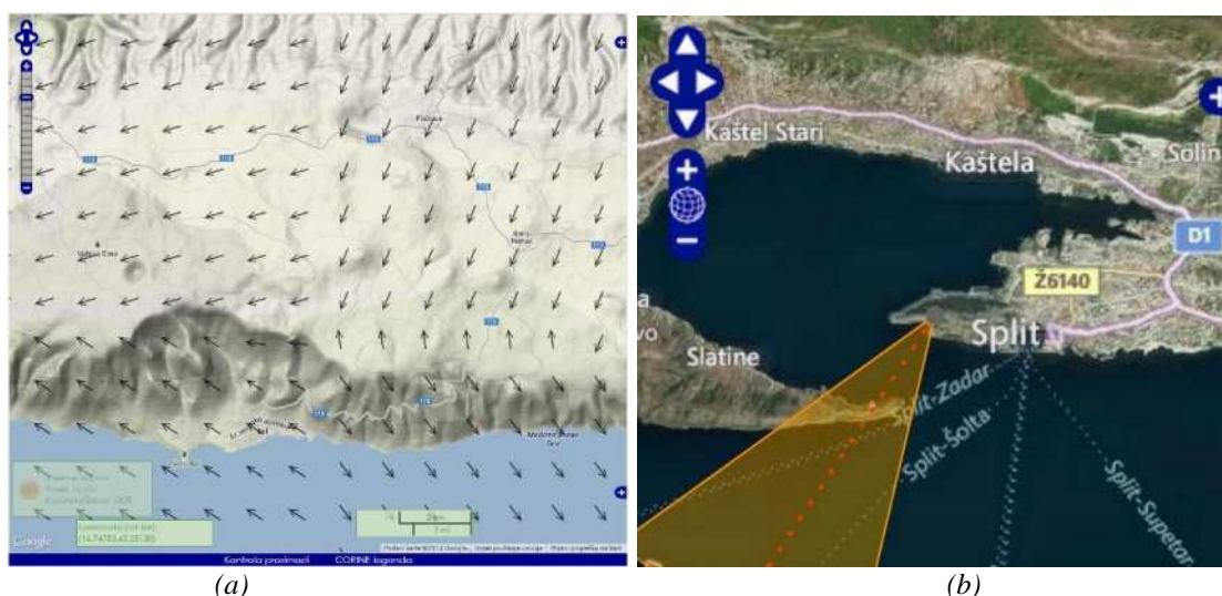
Figure 4. a) Superposition of dynamic meteorological data on GIS maps and b) presentation of cameras azimuth and field of view on GIS map
