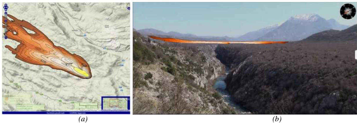
Figure 5. a) Simulated wildfire spread shown on GIS map and b) superimposed in real time on real camera view using Augmented Reality methods
