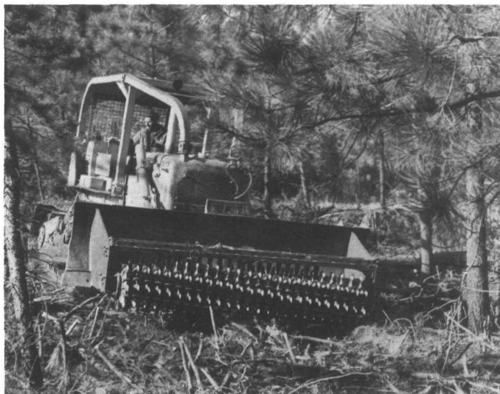
Figure 2.--Tomahawk crusher mounted on crawler tractor crushes slash from thinning of pines.
