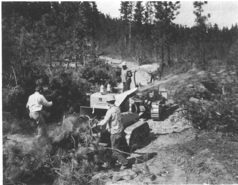
Figure 5.--Chipping logging slash on the Deschutes National Forest. Chipper is being used here to dispose of slash from a thinning, but equipment could also be used in clearcut areas.
