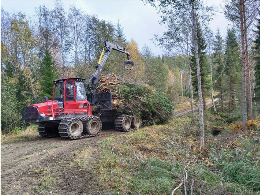
Fig. 25.6 Conventional forwarder loaded with small-diameter trees from a bioenergy thinning operation in Bräcke, northwestern Sweden, October 2019. Photo credit Raul Fernandez Lacruz
