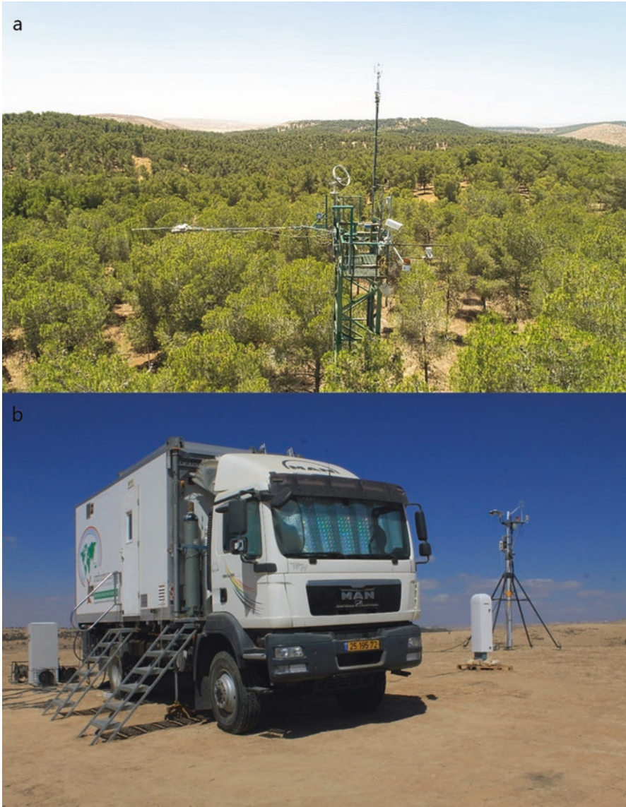
Fig. 14.3 (a) The micrometeorological tower for measuring water, carbon and energy fluxes over Yatir Forest at the Northern edge of the Negev desert in Israel; (b) Mobile laboratory with the pneumatic mast (adjustable up to 28 m) for micrometeorological and flux measurements in the background, during measurements at a desert site 4 km outside the Yatir forest
