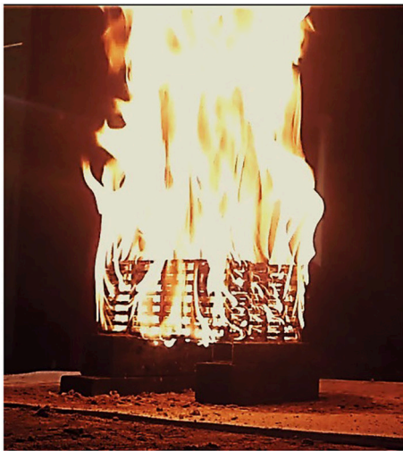
FIGURE 3 | Loosely-packed crib (crib design #11) burning in a quiescent environment showing the entire fuel bed burning uniformly throughout.
