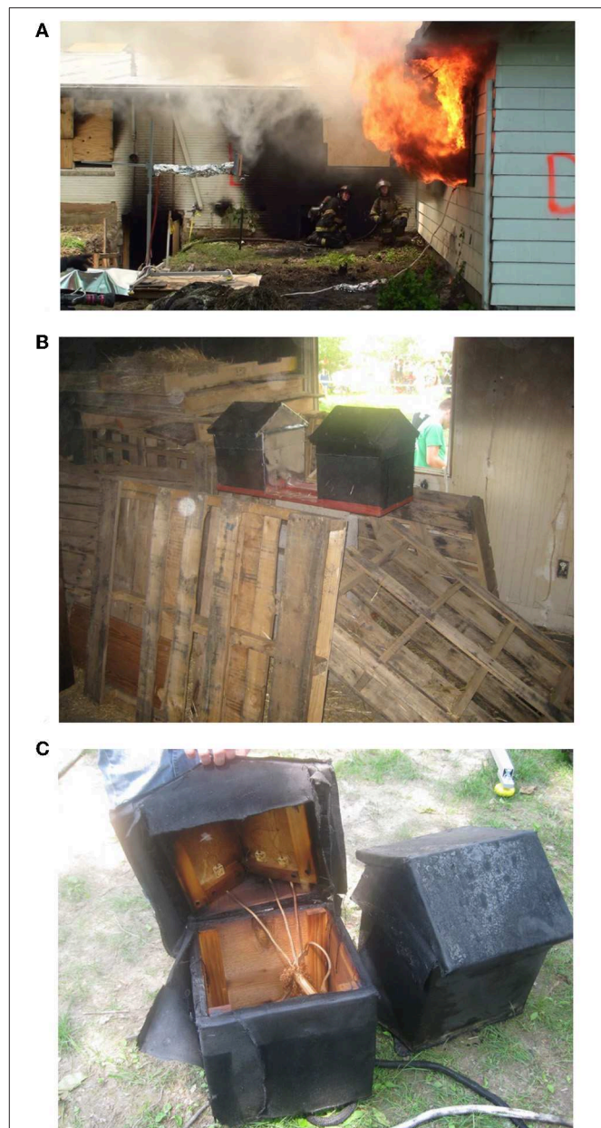
FIGURE 2 | The burn-room experiment in Avon Lake, Ohio experiment. (A) The fire gushes through the window toward a temperature and heat-flux sensor stand (left), (B) the blanketed wooden model structures surrounded by pallets before ignition. Left: metallic polyester coated amorphous silica (AAS1800) and right: pre-oxidized carbon fiber (CK-3), and (C) the structures after fire exposure (left: CK-3 and right: AAS1800).
