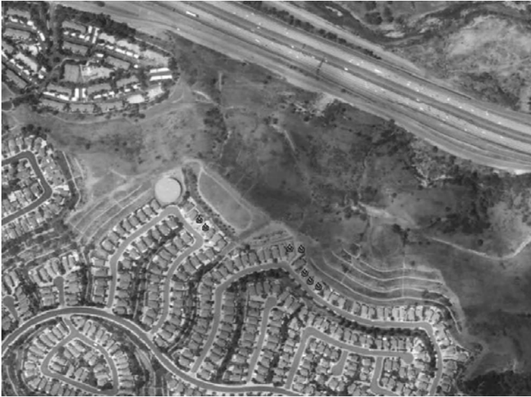
Fig. 13.6 Prefire aerial image of urban housing adjacent to wildlands affected by the 2008 Freeway Fire in southern California. Flames on the seven houses on the upper perimeter indicate they were destroyed by the fire; houses at the WUI on the left have substantial clearance between homes and wildlands and houses on the right had a well-watered greenbelt. (From C.J. Fotheringham & J.E. Keeley unpublished data.)
