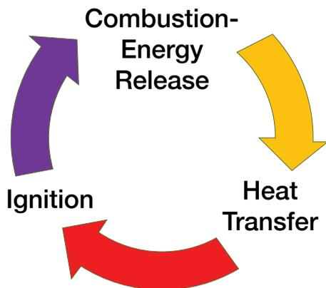
FIGURE 4-5 Cycle of fire spread.
