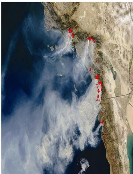
**Figure 4.7** An example of the visible imagery showing the smoke from fires is shown. The red areas indicate the location of fires detected on the 3.9  $\mu\text{m}$  of infrared imagery
